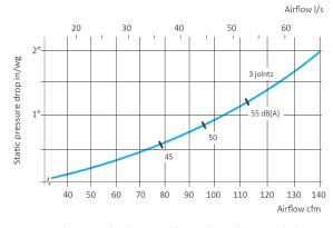
Static pressure drop is measured in accordance with ISO standard 5167-1. The noise level is measured in accordance with ISO standard 3743.
