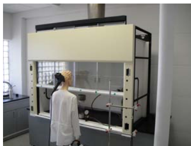
Tracer Gas Test, Center Position
