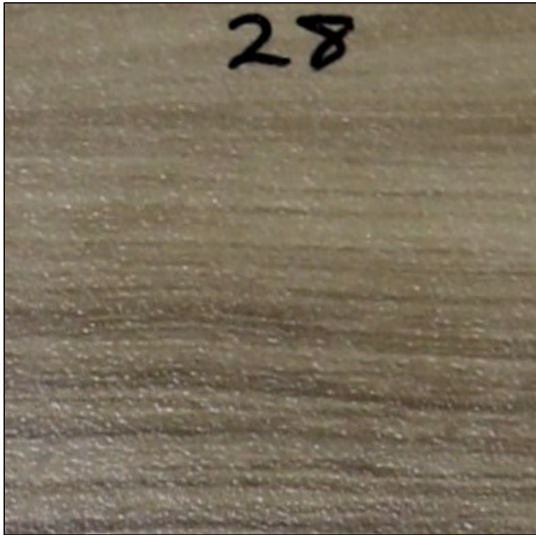
Chemical Spot Test: #28, Methylene Chloride, Rating 2, Gloss change
