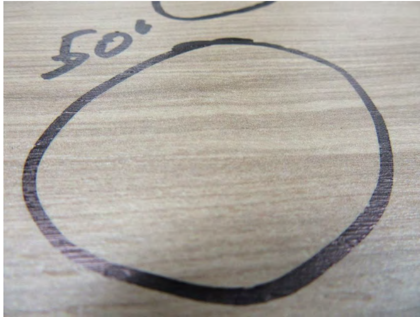
Figure 2: 8.3 Ball Impact Resistance Test no fracturing observed at 50 inches
