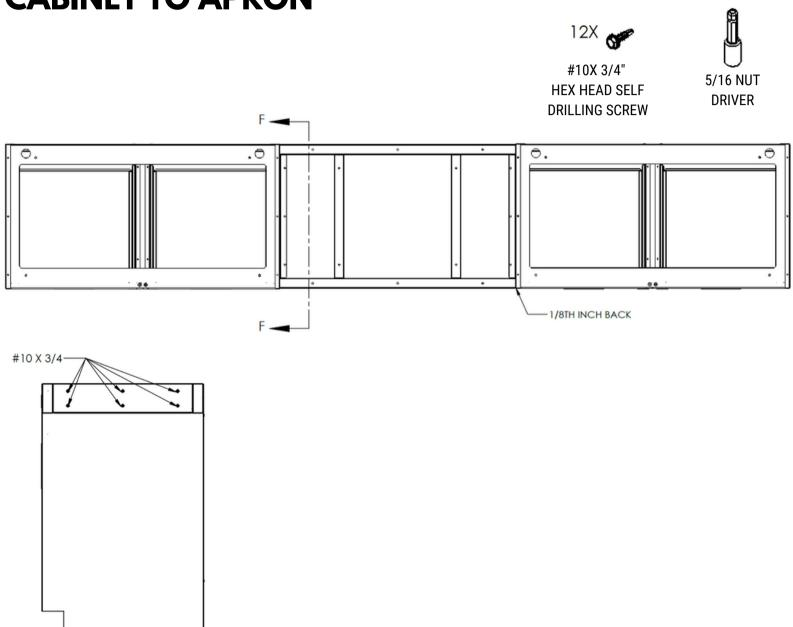
WITH APRON FLUSH ON TOP SLIDE IT BACK ~1/8TH OF AN INCH FROM THE FRONT OF THE CABINET. USING 12 #10 X 3/4 SELF DRILLING SCREWS SECURE THE APRON TO THE CABINETS.
