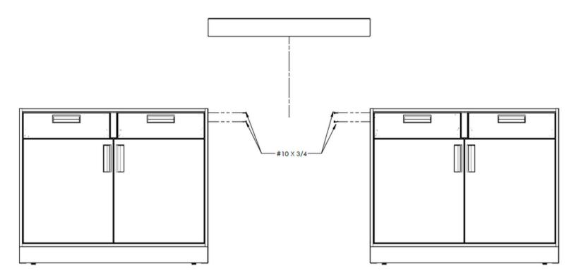
SET AND LEVEL CABINETS ON EITHER SIDE OF APRON, ENSURING GAP BETWEEN CABINETS IS THE WIDTH OF THE APRON. SLIDE APRON IN FROM ABOVE UNTILL IT IS FLUSH ON TOP WITH OTHER CABS.
