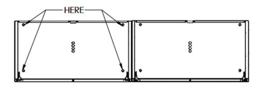
LEVEL CABINETS BY PLACING IMPACT WITH EXTENSION THROUGH THE LEVELER HOLES. RIGHT WILL RAISE LEVELER LEFT WILL LOWER LEVELER
