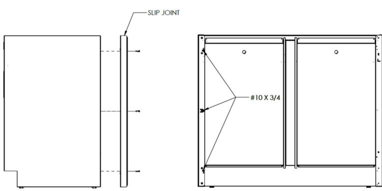
PLACE SLIPJOINT FLUSH WITH TOP AND SIDE OF CABINET USEING THREE #10 X 3/4 SELF DRILLING SCREWS ATTACH SCRIBE TO CABINET
