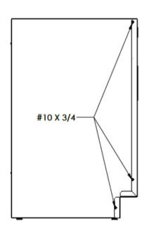
FLUSH FILLER WITH FRONT AND TOP OF CABINET ATTACH USING THREE #10 X 3/4 SELF DRILLING SCREWS
