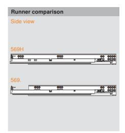
**NOTE:** Material thickness may vary. Inside drawer width **must** equal opening width minus **42** for TANDEM to align and function properly.
