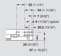
**NOTE:** Elongated holes are for  $\pm 4.5$  (3/16") depth adjustment only. Additional screws must be used to secure the runner to the cabinet.
