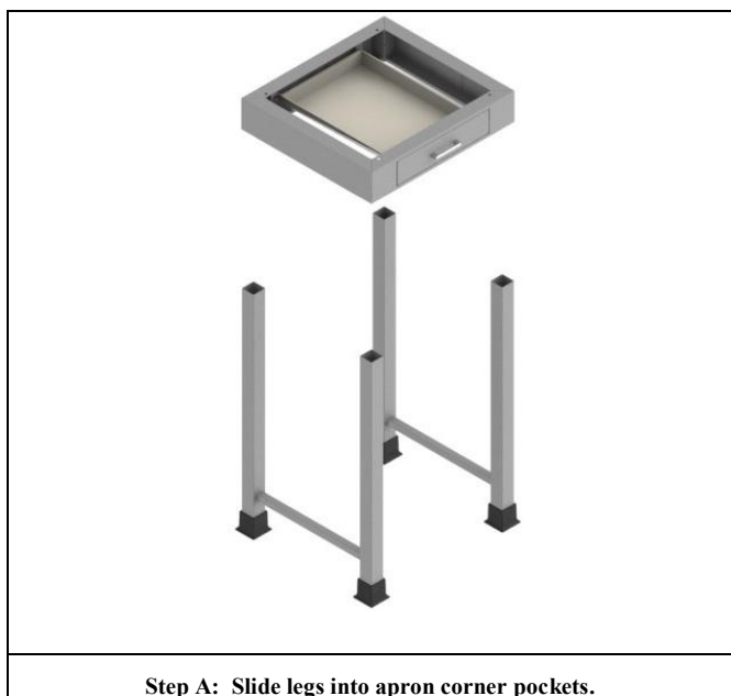
Step A: Slide legs into apron corner pockets.
