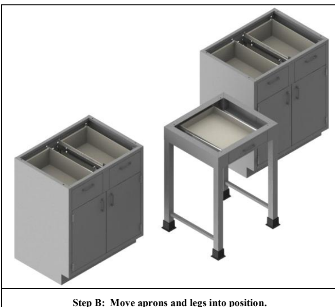
Step B: Move aprons and legs into position.
