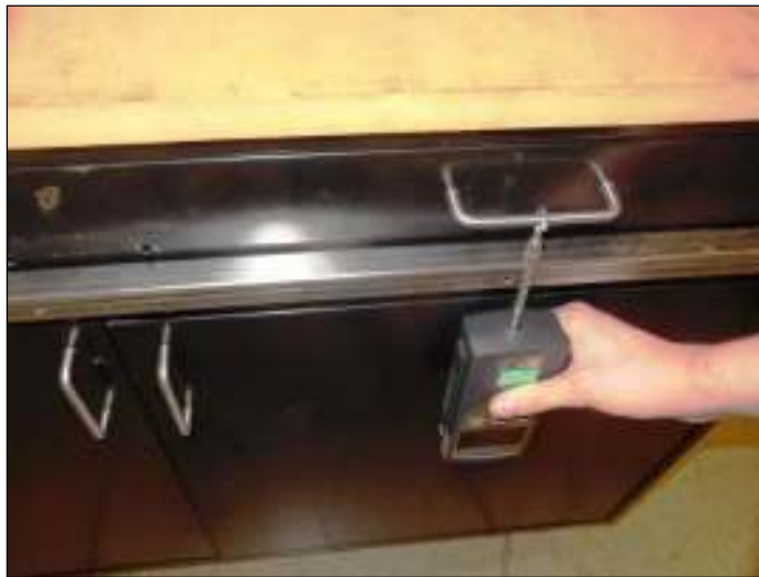
Drawer and Door Pull Test; Drawer Vertical
