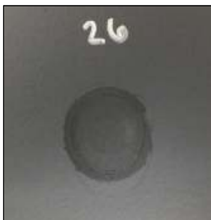
Chemical Spot Test 26 Iodine, Tincture, Rating 2, Staining
