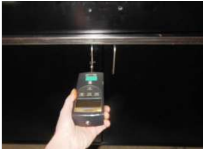
Drawer and Door Pull Test; Door Horizontal
