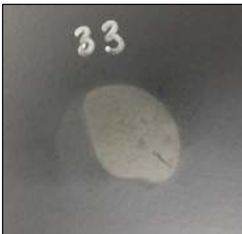
Chemical Spot Test 33 Nitric Acid 70%, Rating 3, Surface Swelling
