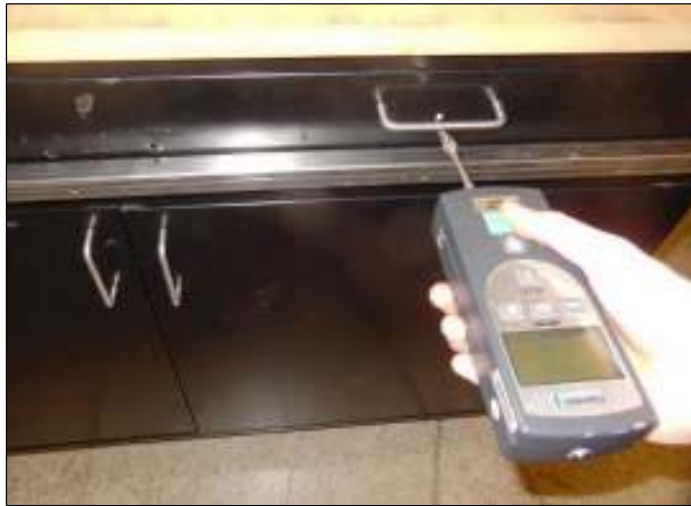
Drawer and Door Pull Test; Drawer Horizontal
