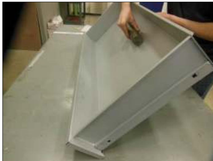
Drawer Internal Impact Test- Rear to Front
