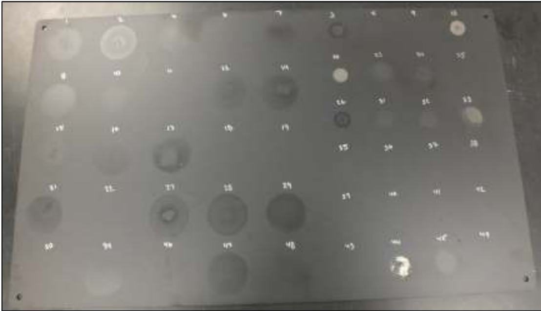
Chemical Spot Test Panel after Exposure
