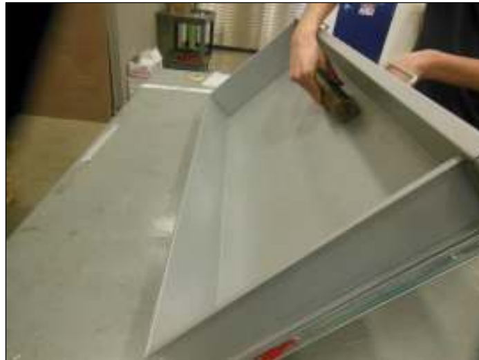
Drawer Internal Impact Test-Front to Rear
