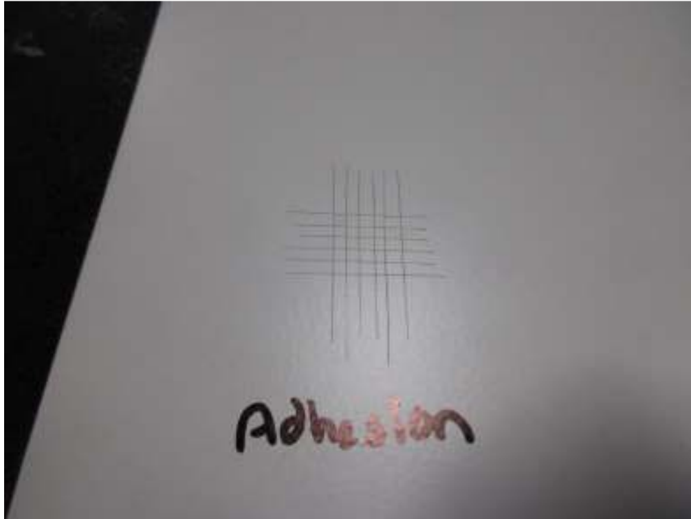
Paint Adhesion on Steel Test after Impact
