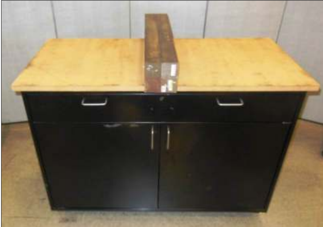
Cabinet Concentrated Load Test
