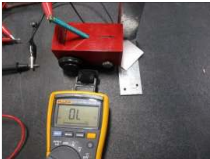
Paint Hardness on Steel Test Set-Up
