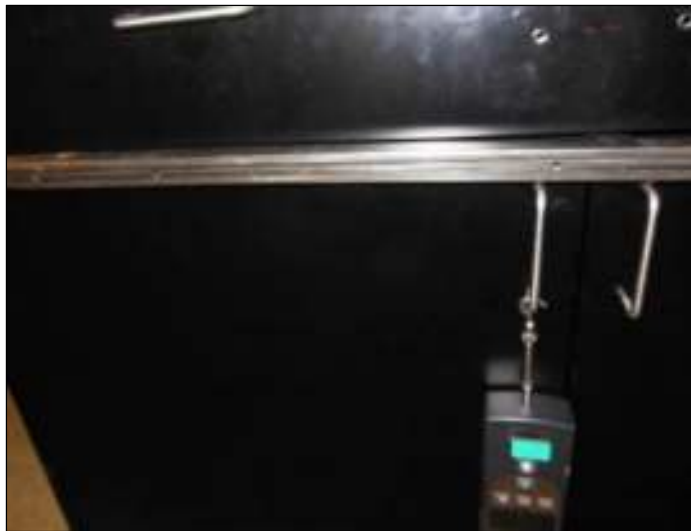
Drawer and Door Pull Test; Door Vertical
