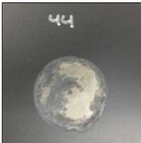
Chemical Spot Test 44 Sulfuric Acid 96%, Rating 3, Surface Erosion
