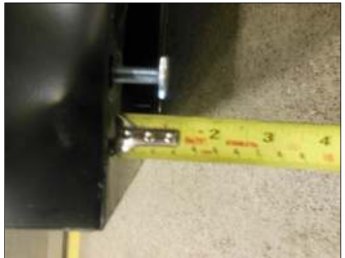
Leveling Bolt Mounted in Cabinet
