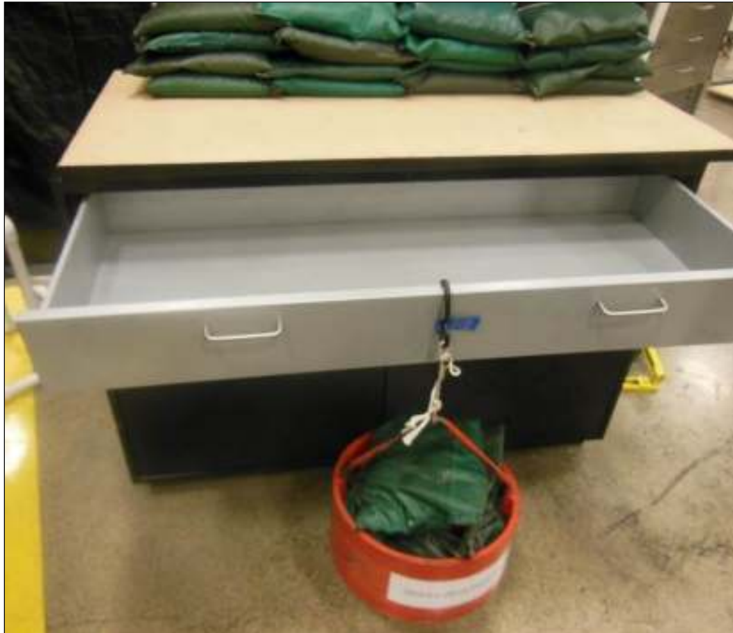
Drawer Static Load Test
