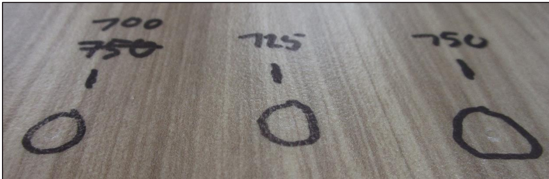
Figure 3: 8.3 Ball Impact Resistance Test Sample After Testing
