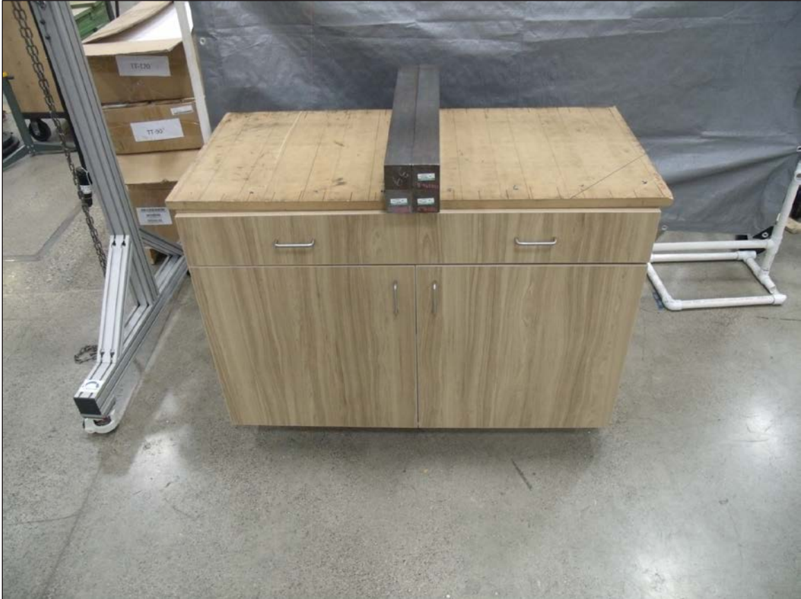
Cabinet Concentrated Load Test
