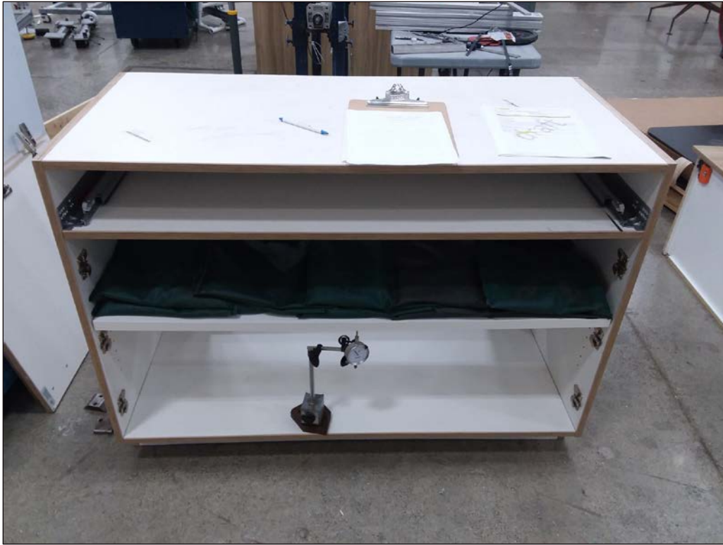
Shelf Load Test – Base Cab
