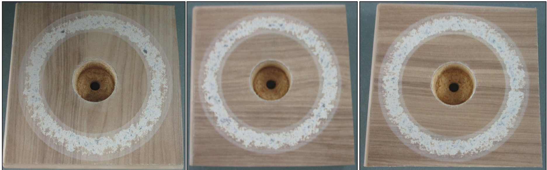
Figure 5: 8.9 Wear Resistance (Abrasion) Samples After Testing.
