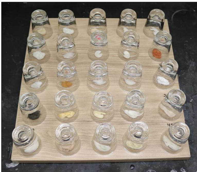
Chemical Spot Test Volatile Chemical Set-up
