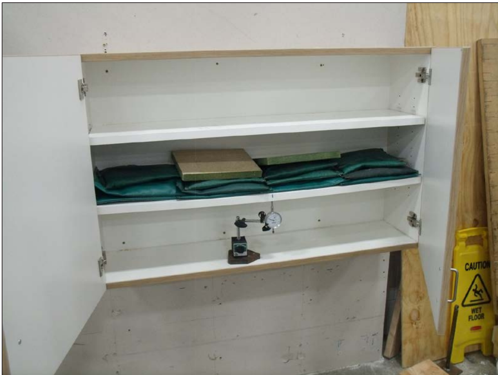
Shelf Load Test – Wall Cabinet
